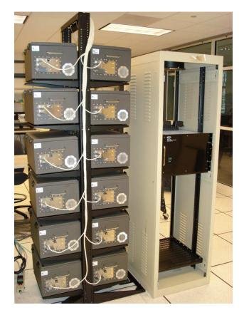
Fig. 2. The MeshTest testbed. The shielded enclosures contain wireless nodes and the RF matrix switch controls the attenuation experienced between the nodes.
