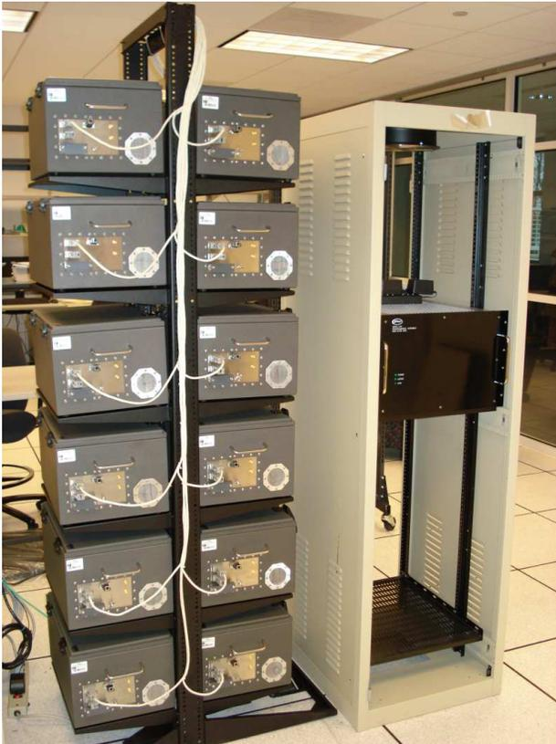
Fig. 2. The MeshTest testbed. The shielded enclosures contain wireless nodes and the RF matrix switch controls the attenuation experienced between the nodes.
